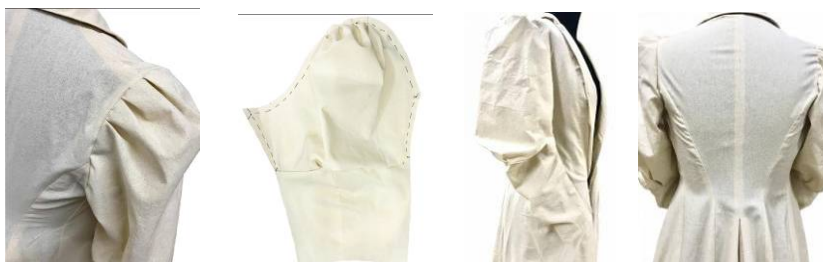
Fig. 6 The box-pleat (a), sewing sleeve lining (b), the sleeve forward state (c), the shoulder line backward (d)
